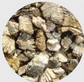
Asbestos Contaminated Vermiculite
