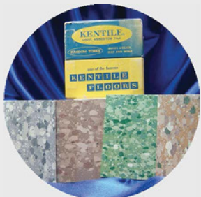
Vinyl Asbestos Floor Tiles
